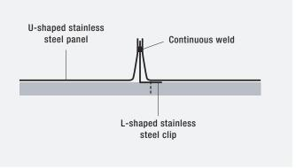
A fully automatic welding machine joins and seals the stainless steel panels. Clips which are anchored to the roof substructure are simultaneously incorporated into the weld.
