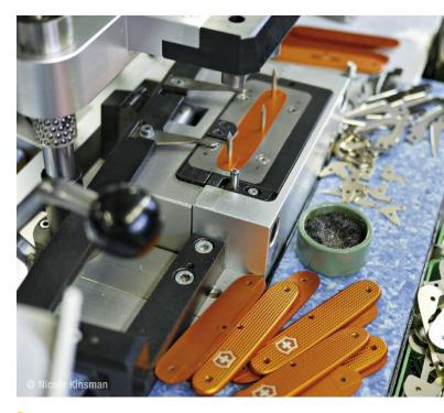
Small-series and custom pocket knives are still assembled by hand. Large-series knives use a fully automated process.
