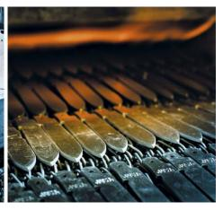
Knife blades are stamped out of a strip of stainless steel, leaving behind scrap to be recycled (left). The raw stainless steel edges are smoothened by tumbling in a deburring machine, filled with abrasive ceramic media (middle). Each blade is heat treated to make it hard yet tough (right). © Victorinox
