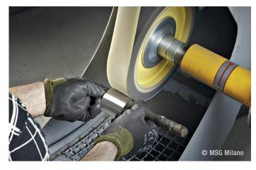
Hand polishing is a step in the production of this stainless steel fitting.
