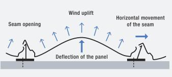
surrounding areas, as well as compromised travel and freight shipment. Fortunately, continuous-seam welded stainless steel roofing provides a solution to both joint damage and roof uplift from wind.
